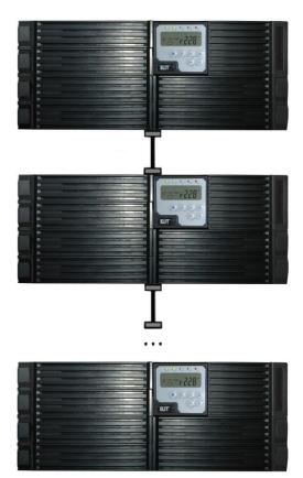
The standard apparatus can be simply interconnected up to 4 units using the CAN-ON (& Alarm Silence) Key bus RJ45 cables on the rear of the SR series UPS. The SR series UPS used an inverter control technology that allows to achieve N+1 scalable redundant power without the use of additional components. Parallel Distribution Box are available till 200 A (40kVA).
